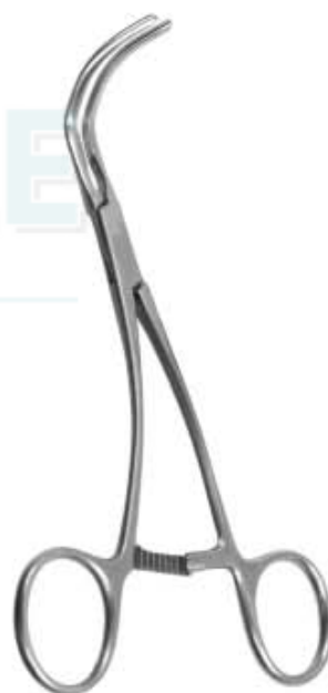
Subramanian "sidewinder" Aorta clamp 9-258-14 14 cm 9-258-16 16 cm jaw length 2.9 cm double curved jaw
